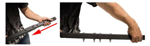
5. Attach the now 97" Horizontal Tube to the 3rd hole up from the bottom of the Metal Leg using one of the  $3/8-16 \times 2.5$ " bolts. Do not tighten. Repeat on all sides.
